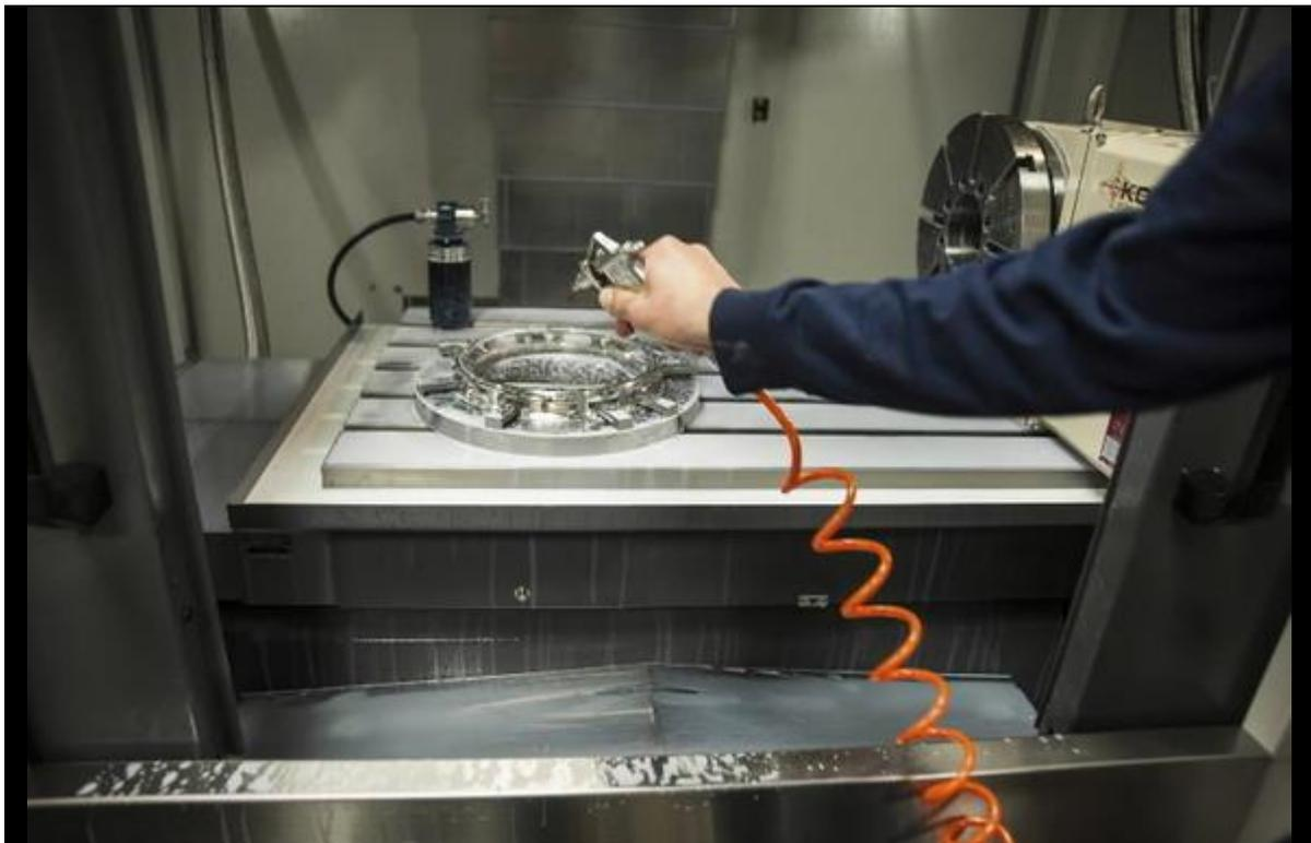
Machinist Douglas Rosen cleans off an Inconel Complex Ring, a hot section jet engine component, at AeroCision, an aerospace engine component manufacturer in Chester, CT on Monday, July 14, 2014. With Rolls-Royce and Honeywell as their major customers, AeroCision is one of a few manufacturers in Connecticut that doesn't sell to Pratt & Whitney. (Daniel Owen / Hartford Courant / July 30, 2014)
